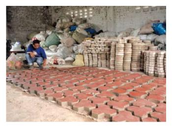
Pavers made from concrete and recovered plastic are used to improve walkways in the city. (photo: Anne Larracas)
